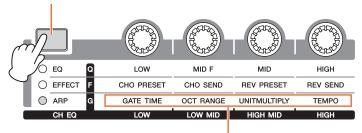
Arpeggio functions controlled via the knobs
