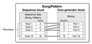
**NOTE** When you play the keyboard in the Mixing mode, the selected Part will not sound, but the Part assigned to the same numbered Track as the selected part will sound, For example, when setting as in the above illustration, playing the keyboard sounds Part 1 even if Part 2 is selected in the Mixing mode.
