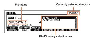
This operation lets you save files to a USB flash memory device. For specific operating procedures, see the Owner's Manual.
