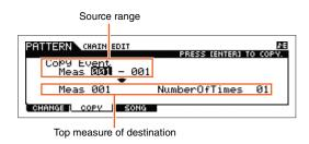
This display lets you copy all Pattern chain events from a specified range of measures (source) to a destination location. After specifying the source range in measures, the top measure of the destination location, and "NumberOfTimes" (number of times the data is copied), press the [ENTER] button to execute the Copy operation.
