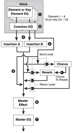
Element EQ applied to each Element (for a Normal Voice) and each Key (for a Drum Voice)
