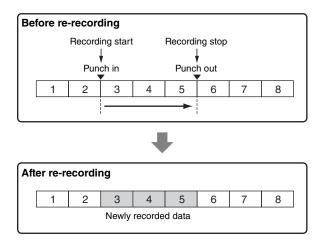
NOTE Punch In/Out Recording can only be used with Realtime recording
