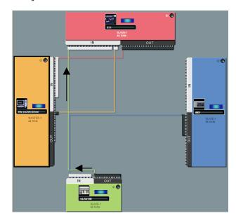
In the above setup we are set to show how the **mLAN16E** can be routed to the 01X on 16 buses (14 + 2). Notice that to follow signal flow the output signal is always the same color as the
