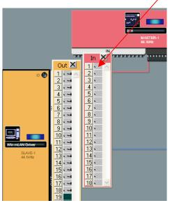
Although only a single line appears to connect the OUT of the computer to the IN of the O1X – it contains all eighteen audio connectors (much like
