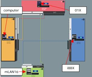
**Breaking a connection:** Place the cursor arrow on the connecting line that runs from the 01X to the computer, it will turn into cross hairs... Right Click and select DISCONNECT ALL or any one of the connections as necessary. If you break a single connection the graphic will adjust and redraw the connections as necessary. Alternatively, when you need to disconnect all – you can click on it and press DELETE.
