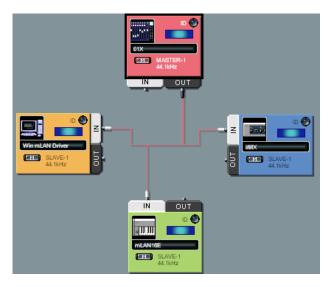
In our setup the 01X is the Master clock. In the diagram above you see the 01X at the top center of the screen shot. It is highlighted (black line outlines the node). You can highlight a node by clicking any where in the colored background within it. To set is as the Master Wordclock:
