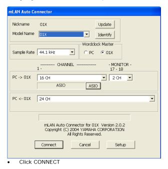
The computer will take a few more seconds to negotiate the setup. If you get a warning that says activate WORDCLOCK on the 01X - do so. This may happen the first time an 01X is powered
