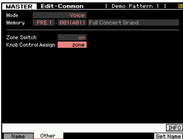
Left: The current MASTER is shown in [EDIT] > [COMMON EDIT] > [F2] OTHER. The MODE is "VOICE", the associated program is PRE 1:001(A01) Full Concert Grand. Because the ZONE SWITCH is ON, this program's Zone parameters will determine how MIDI is transmitted.
