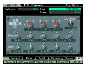
The three brown knobs on the top row are labeled "Q". The second row of five knobs is the "Frequency" setting. The five knobs of the bottom row are the "Gain" boost or cut. In the upper right corner is the overall OUTPUT.
