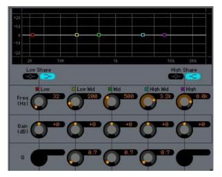
Notice that above the Low and High bands you can select the "Shape" – this selection is between a peaking type or shelving type filter band.
