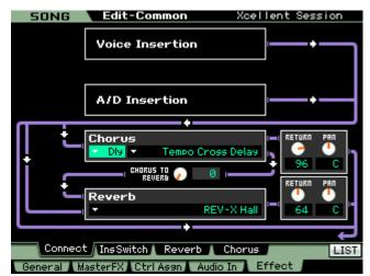
Notice also that both the Performance and Song Mixing screens do not have <u>send</u> level controls *to* the Reverb and Chorus. This is because the send level is not a 'common' parameter but is on a **per** PART basis. **Each** Part will have its own control for the amount of signal sent to the System Effect on the Part Edit level. While in Edit, you can select the PART to edit by touching the Track buttons 1-16 –corresponding to Parts 01-16.
