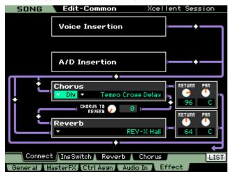
The Tone Generator block can have up to 16 Parts total. The DUAL INSERTION EFFECT can be activated on any eight Parts from the internal XS (1-16). Each Part will have an individual send to the System effects. And finally, all signal goes through the Master EFFECT, the Master EQ and then on to the main stereo outputs.
