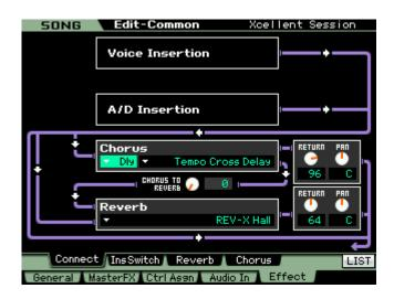
You can drop into edit any of these via the associated [SF] (Sub Function) button. For example, in the screen above [SF3] is Reverb and [SF4] is Chorus.
