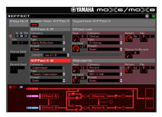
In the screen shot above we see a DRUM KIT Effect routing flow chart (from the MOX6/MOX8 Editor). The "KEY OUT" parameter in the upper left corner indicates we are looking a KEY "C1" (a Kick Drum) which is routed to INSERTION EFFECT B (blue) which is a "Classic Compressor".
