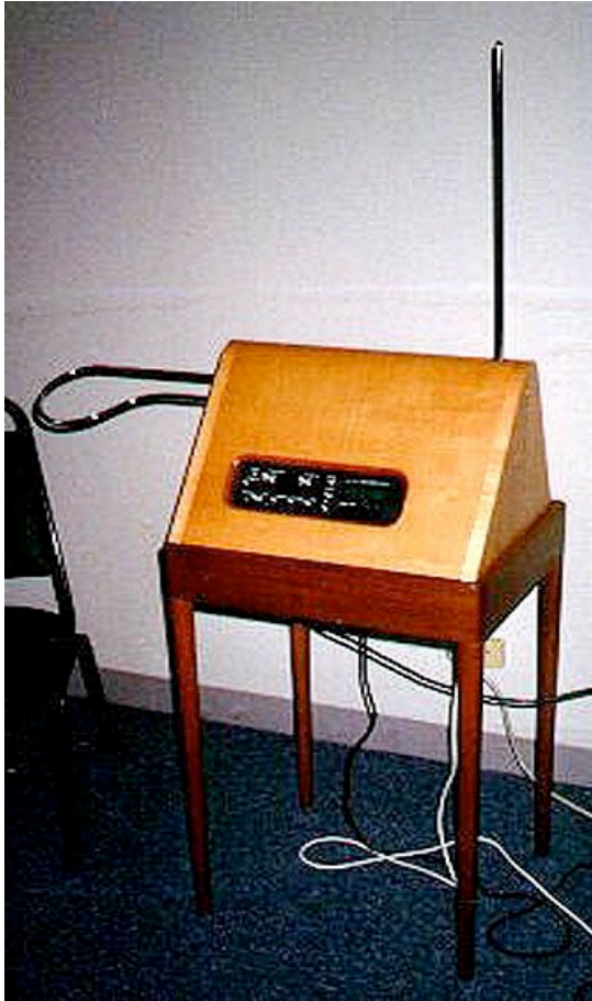
Ethervox Theremin. Note one antennae sticking up, the other antennae laying horizontally on the left.
