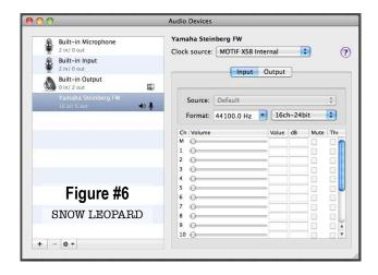
NOTE: The Motif XS and YSFW Driver use 'YSFW Main' (Port 1) to send MIDI to the DAW (Logic Pro 9) and from the DAW (MIDI tracks) to the Motif's tone generator... 'YSFW MIDI OUT' is used as a MIDI thru channel. It is used to utilize an external synth physically connected to the XS' MIDI Out. 'YSFW Remote' is used to control the DAW from the Motif. A final port, which is not visible from within Logic, is used to simultaneously utilize the Studio Manager / XS Editor as a stand alone...
