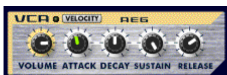
Fig. 6. The VCA envelope generator attack and release times are increased to get a voice with slow amplitude rise and fall in note-on and note-off.
