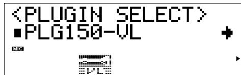
(If necessary) Press SELECT button to place the cursor to PLG150-VL.
