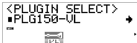
(If necessary) Press SELECT button to place the cursor at PLG150-VL.
