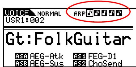
You can change the active arpeggio in real time by pressing the PAGE [<]/[>] buttons on the front panel. Or you can assign a MIDI controller to do the job. For this example, place this Voice in an initialized Multi – as **PART01** (shown below)
